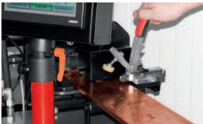
Holdfast for the busbars during cutting.
