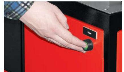
Control key for cutting busbars.
